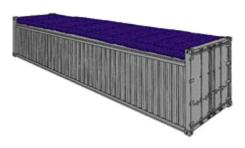
For large and/or high pieces that can not be loaded through container doors, such as machineries, marble, glass sheets, etc
